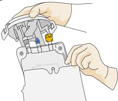
**2A:** Turn off vacuum. Open and completely remove lid to expose PUREGRAFT filtration bag.
