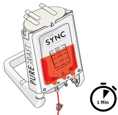
**2C:** Hang PUREGRAFT filtration bag from hook and allow waste fluid to drain for **1-3 minutes** (or until fluid stops draining).
