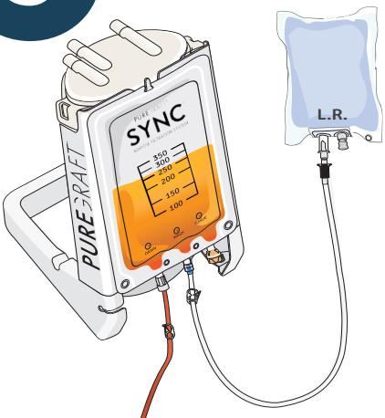
**3A:** Close DRAIN clamp. Connect irrigation tubing to WASH port and add 200mL Lactated Ringer's (LR) solution.
