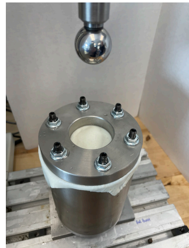
Figure 5: Puregraft Essence fixed within Ball Burst test fixture
